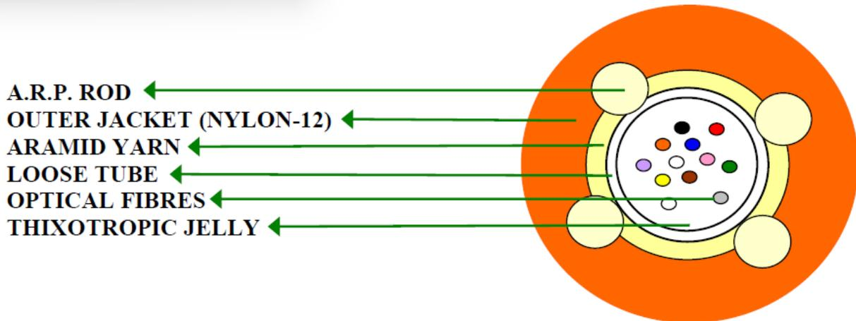
**3.8.4 Filling compound** : The filling compound used in the loose tube shall be compatible to fibre and secondary protection of fibre ~~ete~~ of the cable. The drip point shall not be lower than +70 ~~degree~~ °C. The fibre movement shall not be constrained by stickiness and shall be easily removable for splicing. Reference
