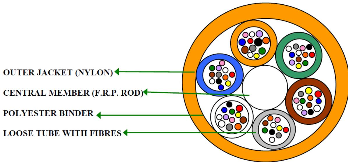
**3.9.3 Strength Member** : Solid FRP non-metallic strength member ~~(FRP)~~ shall be provided in the center of the cable core. The strength member ~~(as per Annexure-#)~~ in the cable shall be for strength and flexibility to the cable and shall have anti buckling properties. The FRP shall keep the fibre strain within permissible values. The strength member(FRP) shall be as per the Standard No. TEC 89010:2021(or latest release) and the subsequent amendments, if any. The size
